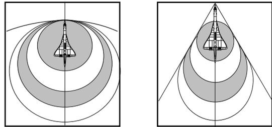
and forms a shock wave. So, if an airplane were traveling toward you at the speed of sound, you would not hear it coming. That's because the sound it makes is traveling at the same speed as the plane itself. If that same plane flew toward you at a speed faster than the speed of sound, you would not hear it until after it had passed.
