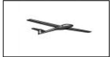
aircraft fly between 100 and 350 mph. These vehicles are usually airplanes with straight, thick wings. This category includes sailplanes, biplanes, propeller planes, helicopters and autogyros. Early German-made planes like the Fokker and the Junkers are in this category. Small planes, like the modern Cessna and Beechcraft, are also grouped within this speed regime.
