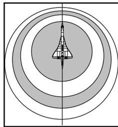
However, when an airplane moves faster than the speed of sound, the air doesn't have enough time to get out of the way. Instead, it piles up in front of the airplane
