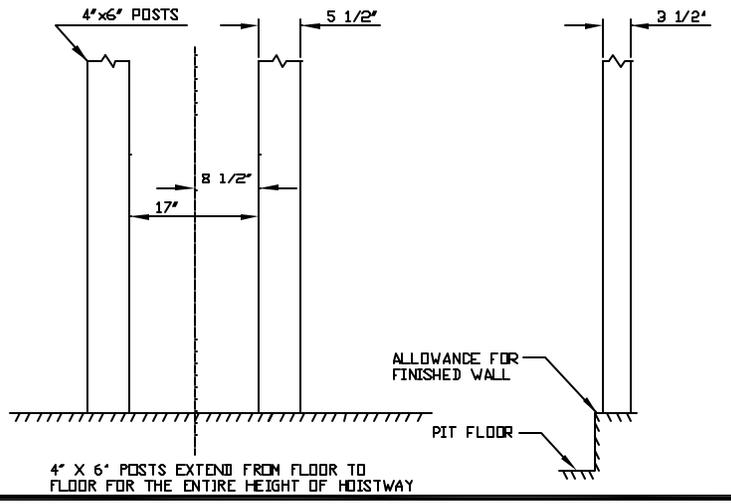
4" X 6" POSTS EXTEND FROM FLOOR TO FLOOR FOR THE ENTIRE HEIGHT OF HOISTWAY
