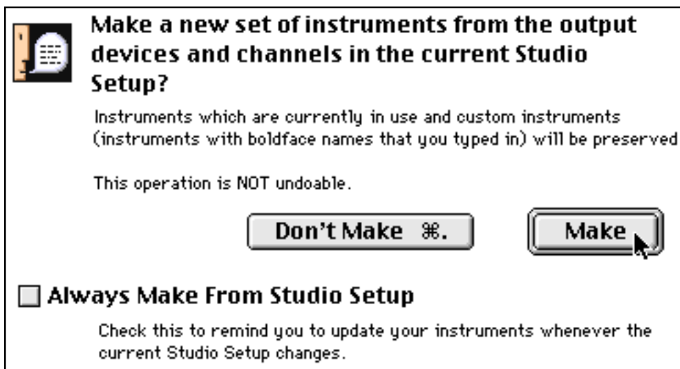
Figure 4.4.4. The Make from Studio Setup command automatically creates output devices based on the current OMS Studio Setup.
