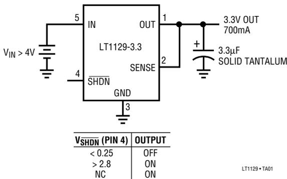
The LT1129-3.3 low dropout linear regulator provides more output current (to 700mA) with only a slight increase in quiescent current (50µA).
