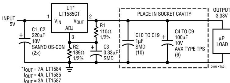
Linear regulator circuits provide simple solutions with superior transient performance for desktop resident Pentium processor-based systems
