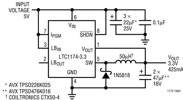
The LTC<sup>®</sup>1174-3.3 current mode DC/DC converter provides efficiencies better than 90% over a wide load current range while requiring only 1µA in Shutdown.
