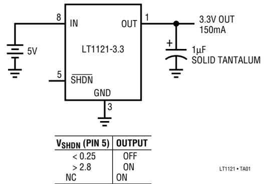
The LT1121-3.3 low dropout linear regulator provides up to 150mA output current with 30µA quiescent current.
