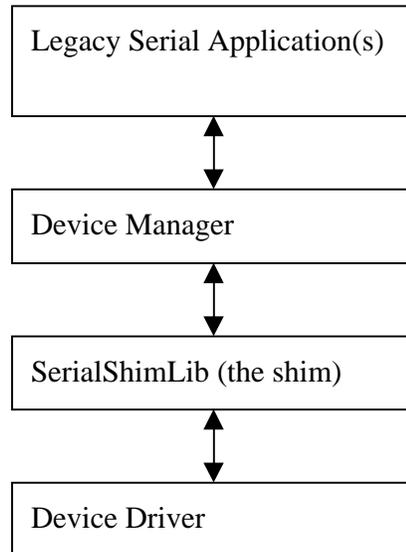
The terms shim, serial shim and SerialShimLib are synonymous and refer to the thin layer that provides the abstraction from the Device Manager and the Communications ToolBox Resource Manager (CRM). The term driver and Device Driver refer to the actual driver that controls the hardware or interfaces to the underlying hardware.
