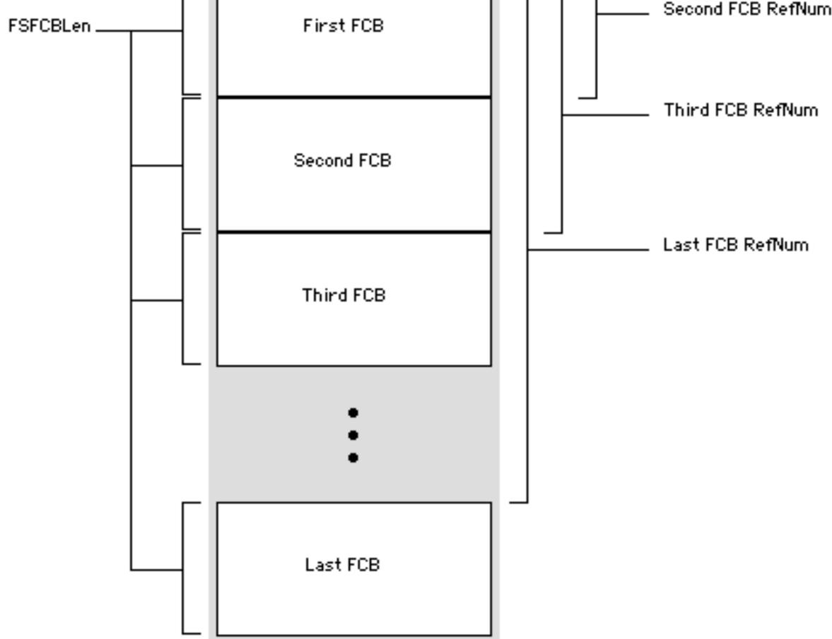
A file reference number is the offset into this table of the corresponding FCB. The file reference number for the 'Nth file is  $2 + (N - 1) * FSFCBLen$ , which yields the sequence 2, 96, 190, 284, and so on.
