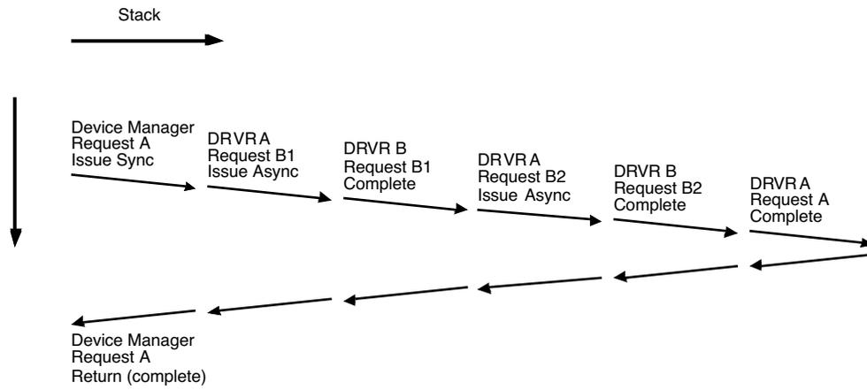
**Figure 2** A driver called asynchronously, calling a synchronous driver.
