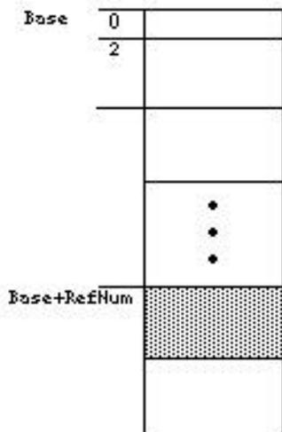
Base is merely the address of the nonrelocatable block that is the FCB buffer. FCBSPtr points to it. The RefNum (a number like \$1D8) is added to Base, to give an address in the block. That address is what the file system will use to read and write to an open file, which is why you are required to pass the RefNum to the PRead and PWrite calls. So RefNum is merely an offset into the buffer.
