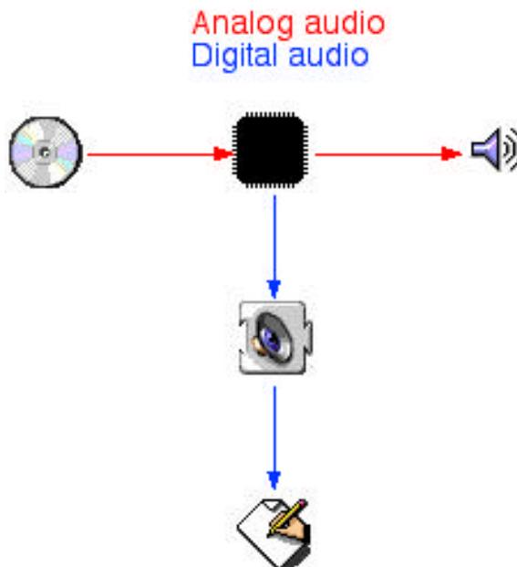
The audio data was read by the CD-ROM drive and converted to analog audio inside the CD-ROM drive. From there the analog audio would go to the sound hardware on the Macintosh. It would then be converted back to digital data and given to the Sound Manager. The Sound Manager would then pass the audio to any application that was recording the CD audio input source. If play through was turned on, the
