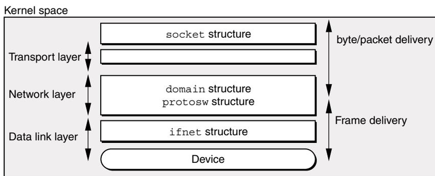
Above the network layer, packets are isolated on a per-user (per-file descriptor) basis. That is, packets are isolated based upon their ownership. Below the network layer, packets are isolated based on which device they go to (or originate from). The network layer provides a transition in how packets are viewed and processed. In the protocol stack (network layer) and the data link layer, the point of view is per-packet. Above these, in the `socket` structure, the point of view is the stream.
