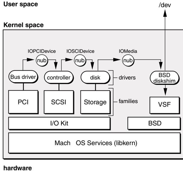
In this example, a connection is made that spans from a disk back to the PCI bus. The connection is made in several steps.
