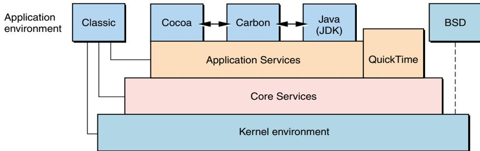
The kernel provides many enhancements for Mac OS X. These include **preemption**, **memory protection**, enhanced performance, improved networking facilities, support for both Macintosh (Extended and Standard) and non-Macintosh (UFS, ISO 9660) file systems, object-oriented APIs, and more. Two of these features, preemption and memory protection, lead to a more robust environment.
