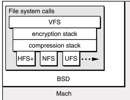
When writing a VFS stack, the developer must create a stub for each vnode operation. In some cases, the stub will simply call the routine of the same name in the underlying layer. Note that stacks may be implemented directly on top of a file system or on top of other stacks, so a developer cannot be sure exactly what the underlying layer will do with a given VFS or VOP call.
