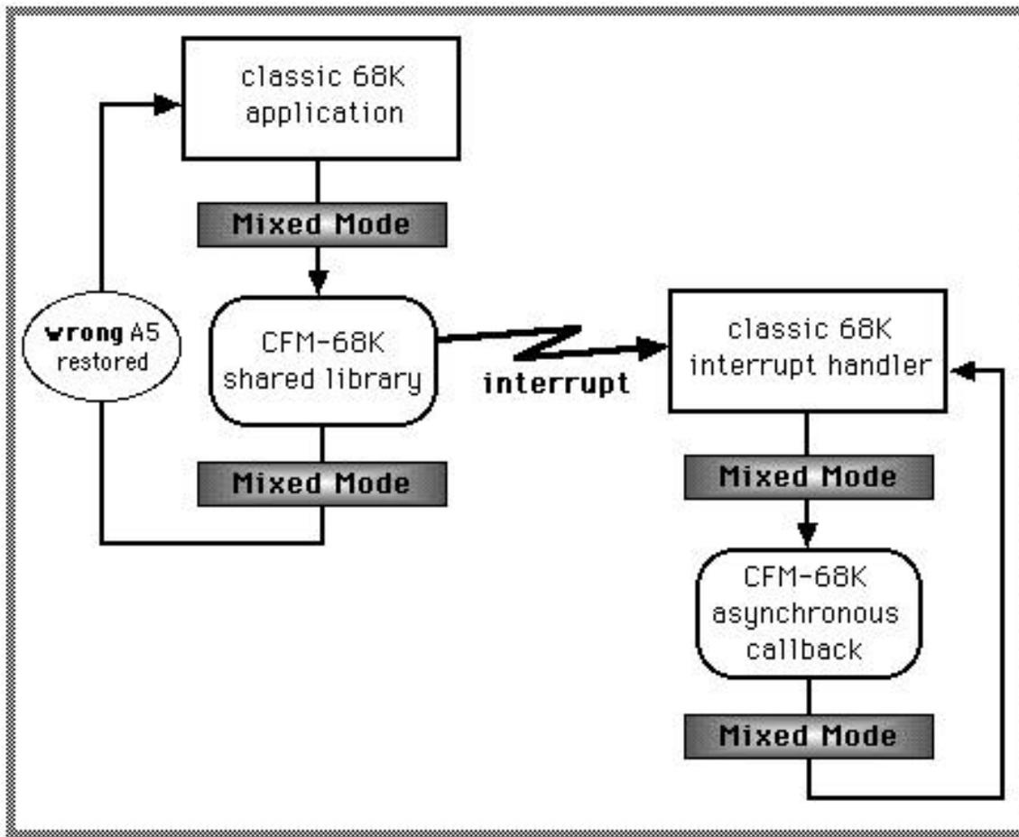
In this example, a classic 68K application calls a routine in a CFM-68K shared library. In order to do so, it must go through Mixed Mode. The CFM-68K code installs an asynchronous callback routine (also written in CFM-68K code). The CFM-68K code gets interrupted and the interrupt handler calls the user's callback routine.
