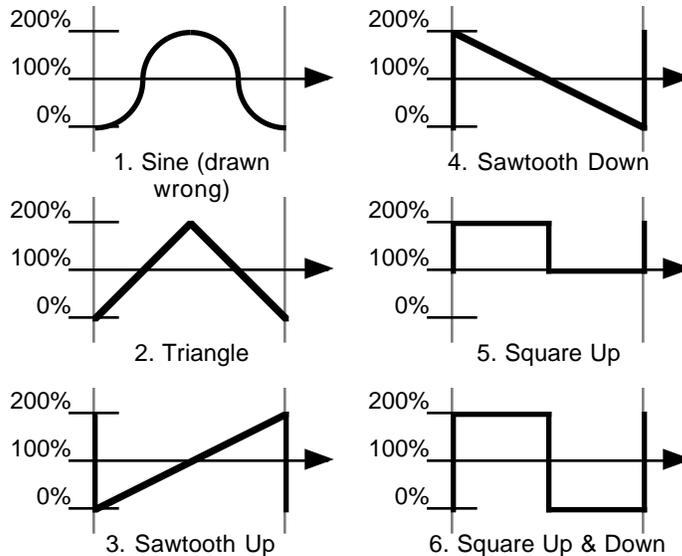
The LFO effect does not necessarily apply to the entire duration of the sound. It can be controlled further by the “Volume LFO Delay” and “Volume LFO Rampup” times. The delay specified in milliseconds a duration before any LFO is applied at all. The rampup time specifies how long it takes to go from no affect to the full depth specified. Thus, the overall volume envelope, including ADSR and LFO parameters, may resemble the following illustration.
