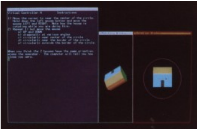
Figure 4. Photo of actual experimental screen of the IRIS. Instructions for each controller are presented on the left, the house orientation to be matched in the middle window, and the house to be rotated in the right window.
