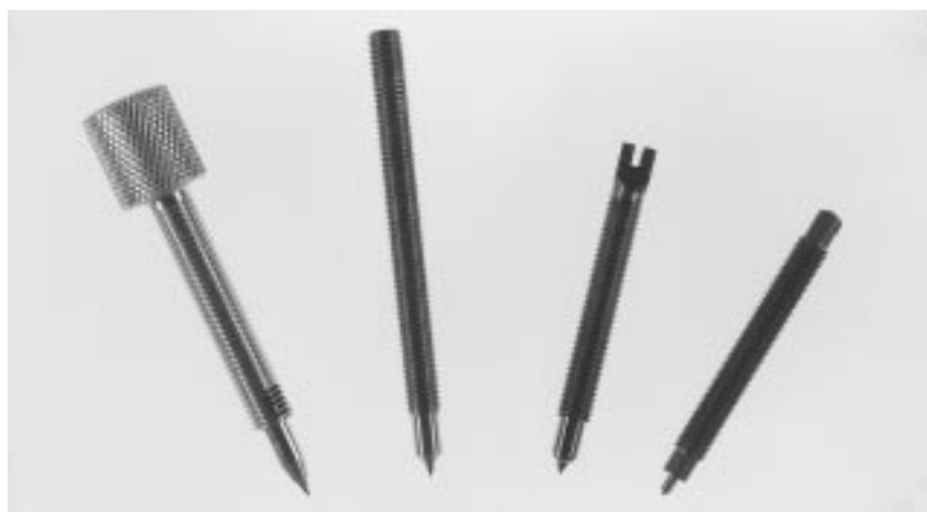
Fig. 2 Various pin designs. On the far left is a Gardner-Wells-type halo pin, with a built-in pressure-sensing device to signal adequate insertion pressure. The two central pins are standard, commercially available halo pins with a broad shoulder. These pins are made of anodized stainless steel. The pin on the far right is an experimental design with a peg-type tip. Preliminary studies show this pin, which is not yet commercially available, and others to have potentially improved biomechanical properties for skull fixation.
