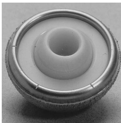
Fig. 2 The Secur-Fit hydroxyapatite press-fit ceramic-on-ceramic bearing prosthesis (Osteonics; Allendale, NJ) has a ceramic articulation that attaches to a metal acetabular shell through a taper lock. It is the only ceramic-on-ceramic bearing undergoing clinical trials in the United States and is strictly for investigational use.
