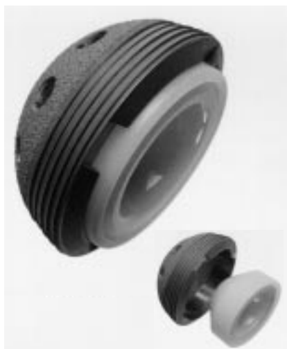
Fig. 3 Left, The Contact acetabular cup design has a ceramic articulating surface fitted into a nonarticulating polyethylene liner, which is then fitted onto a metal acetabular shell. This design is not currently available in the United States. Above, Cross section through the Contact acetabular cup. UHMWPE = ultra-high-molecular-weight polyethylene. (Courtesy of Paolo Dalla Pria, MD, Lima-LTO, Casiasco PN, Italy.)
