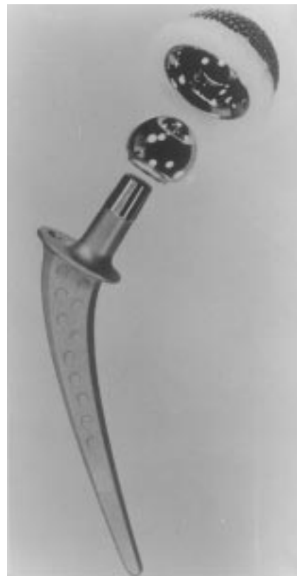
Fig. 4 Weber THA prosthesis consists of a modular titanium cemented femoral stem with a curved or straight design and a four-layer sintered stainless-steel mesh cup. The articulation consists of a 28-mm CoCrMo alloy femoral head and a CoCrMo metal shell fixed within an outer polyethylene cup. This device is strictly for investigational use and is not available in the United States. (Courtesy of Weber BG: Experience with the Metasul total hip bearing system. Clin Orthop 1996;329[suppl]: S69-S77.)
