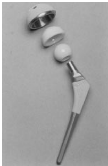
Fig. 2 The Secur-Fit hydroxyapatite press-fit ceramic-on-ceramic bearing prosthesis (Osteonics; Allendale, NJ) has a ceramic articulation that attaches to a metal acetabular shell through a taper lock. It is the only ceramic-on-ceramic bearing undergoing clinical trials in the United States and is strictly for investigational use.
