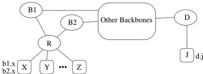
It is important to note that if the source address on the outgoing NPDU has prefix B2, then the resulting incoming NPDU will return via backbone B2 (assuming that, for scaling purposes, B2 advertises only prefix B2, and X's B2-based prefix is not advertised through B1).
