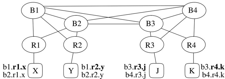
go through B3, but will not necessarily go through B1 (depending on whether R1 chose B1 or B2 for its path to B3). Therefore, it is necessary for X (or R1 or B1) to install an SA-route for X. With the SA-route, NPDUs would go through B1 on the way to J, and would return through B1 on the return path because the ES in J would put the source address of the incoming NPDU into the destination address field of the outgoing NPDU.
