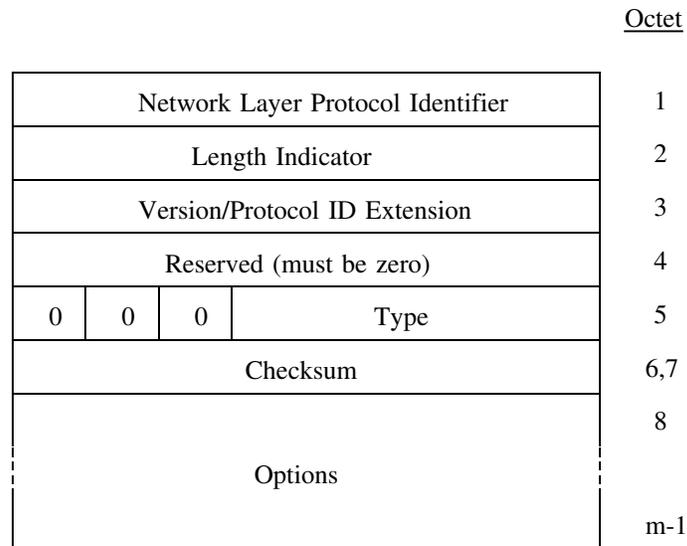
**Figure 13: RA PDU Format**
