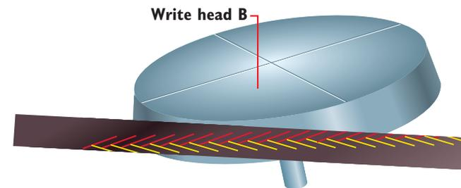
**5** As write head B passes over the tape, it writes data in a track at a 40-degree angle to track A, making a crisscross pattern that overlaps track A. The overlapping data packs more information per inch of tape; it isn't misread later because the magnetic bits written by the two write heads have different polarities, and the different read heads read data only from properly aligned tracks.
