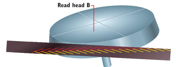
**6** Read head B and write head B go through the same steps, alternating with the A heads until all the data is backed up. Then the drive rewinds the tape and writes a directory of stored files either in a special partition at the front of the tape or in a file on the hard disk.
