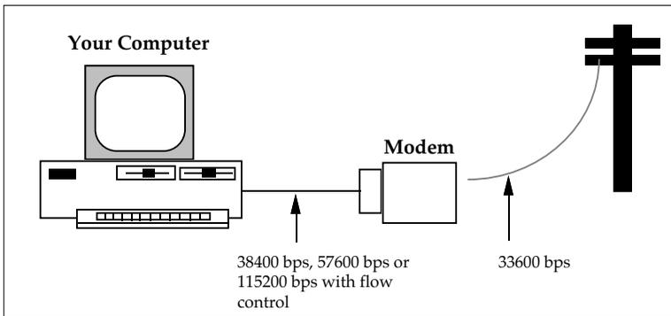
☞ For communications above 19,200 bps, a 16550 serial card is required.
