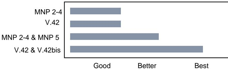
If you are connecting to various makes and models of modems, V.42/V.42bis auto-reliable mode is probably the best alternative (**default**). V.42/V.42bis auto-reliable mode will also connect to another modem that supports MNP with V.42bis data compression. For overseas or cellular connections, use MNP 10 or MNP10EC if possible.
