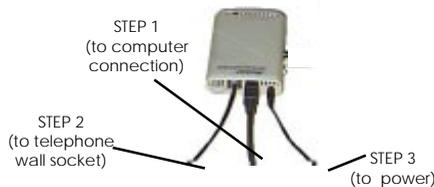
2. Plug the smaller end of the telephone cable into the **Line** socket at the back of your modem and the other end into your telephone line socket on the wall.
