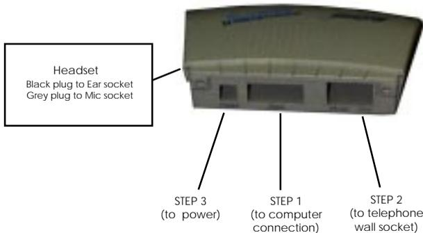
2. Plug the smaller end of the telephone cable into the **Line** socket at the back of your modem and the other end into your telephone line socket on the wall.
