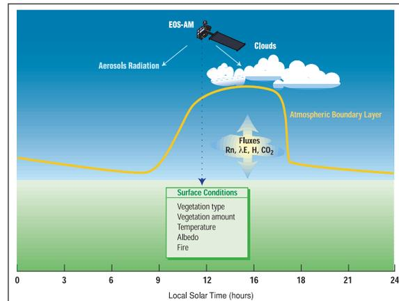
AM-1 Platform diagram showing types of measurements made from the EOS AM-1 satellite platform that will contribute to parameterization and testing of land-surface models. Note that the morning equatorial overpass will improve measurements of surface conditions by avoiding interference from afternoon convective clouds.
