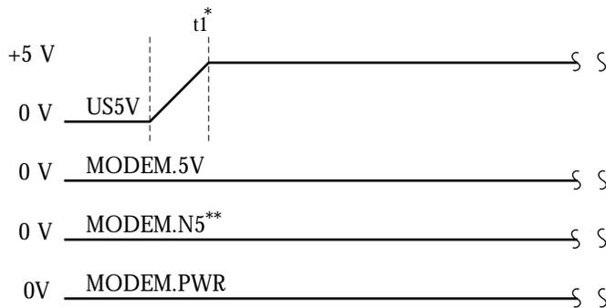
\*  $t1 = 2$  ms (typical), 30 ms (maximum). After  $t1$ , maximum overshoot is less than 50 mV peak to peak.
