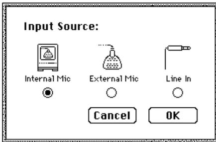
Either the external microphone or line-level inputs can be plugged into the sound input jack. When the user selects the corresponding input device in the Sound control panel, the computer sets the gain appropriately.
