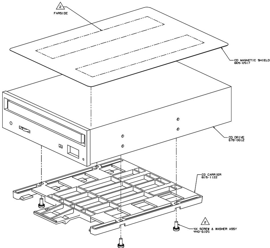
Foldout 2 is a design guide for the sled used for a 5.25-inch device in the Macintosh Centris 610 and Macintosh Quadra 800 computers.
