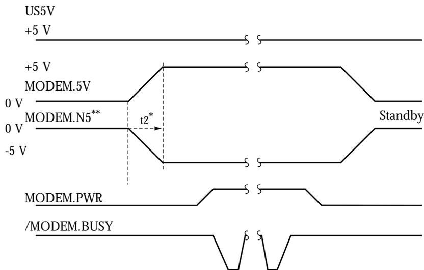
\*  $t2 = 35$  ms (typical), 70 ms (maximum). After  $t2$ , maximum overshoot is less than 50 mV peak to peak.
