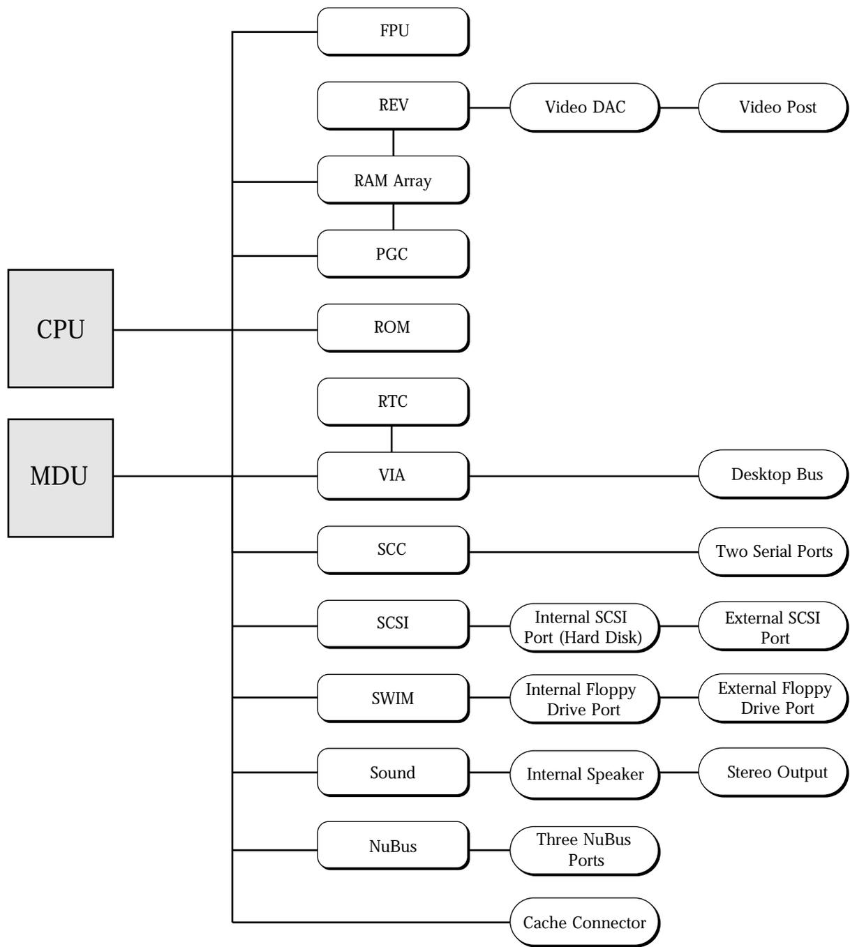
• **Figure 1-2** Hardware block diagram
