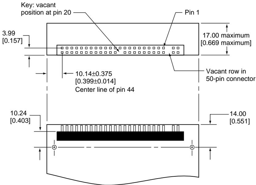
Note: Dimensions are in millimeters [inches].
