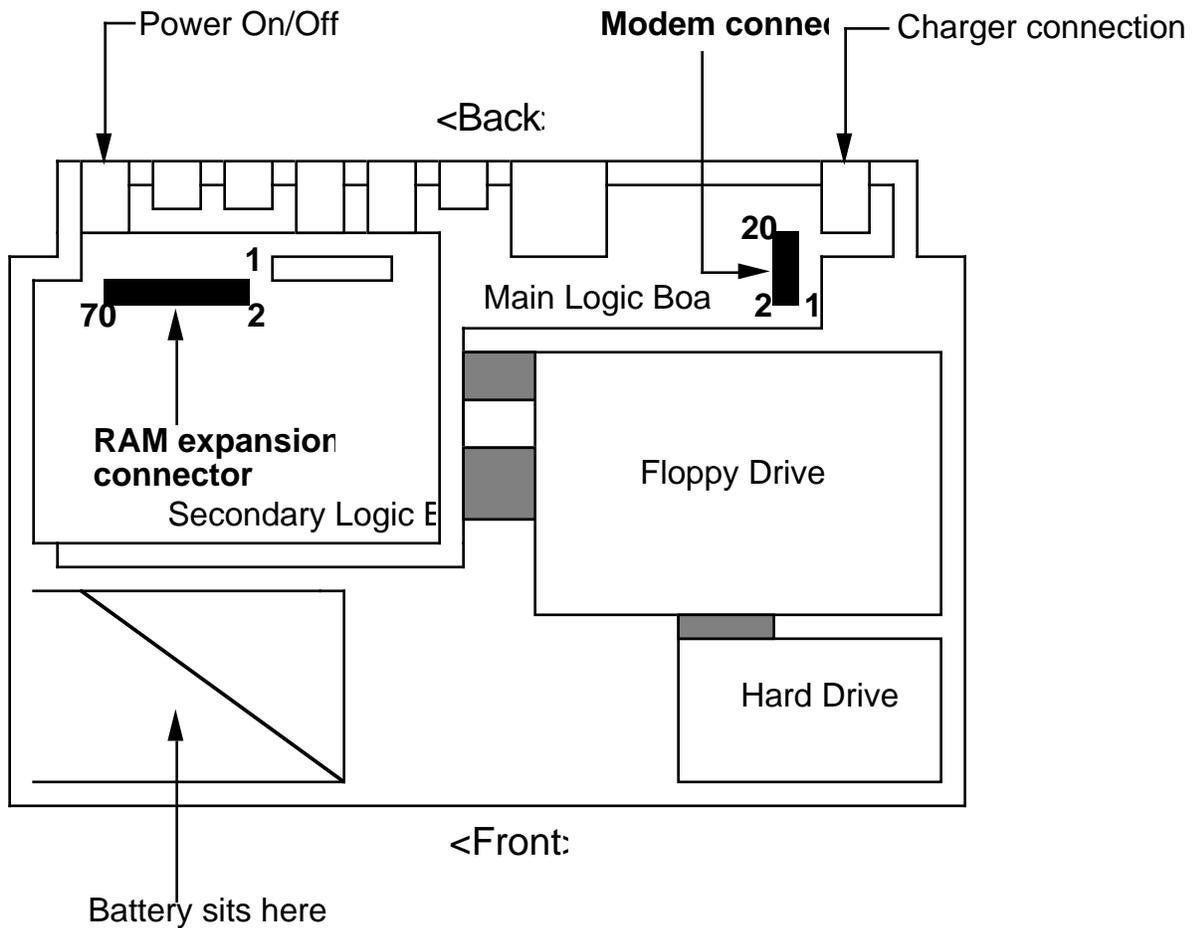
As is the case with the permanent ROM, only 4-Mbit chips are used for expansion RAM. For example, a 4 MB RAM expansion card has eight 4-Mbit PSRAMs (512K x 8-bit chips arranged as two banks of 32 bits), and a 6 MB card has twelve 4-Mbit PSRAMs (512K x 8-bit chips arranged as three banks of 32 bits). Access and cycle times for these devices are 100 ns.
