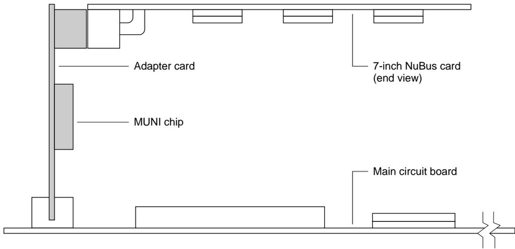
The MUNI (Macintosh Universal NuBus Interface) chip shown in Figure 1-1 mediates between NuBus and the MC68040 processor bus.
