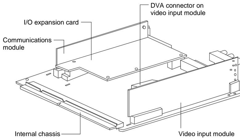
Figure 4-5 shows the orientation of the DVA connector on the video input module.
