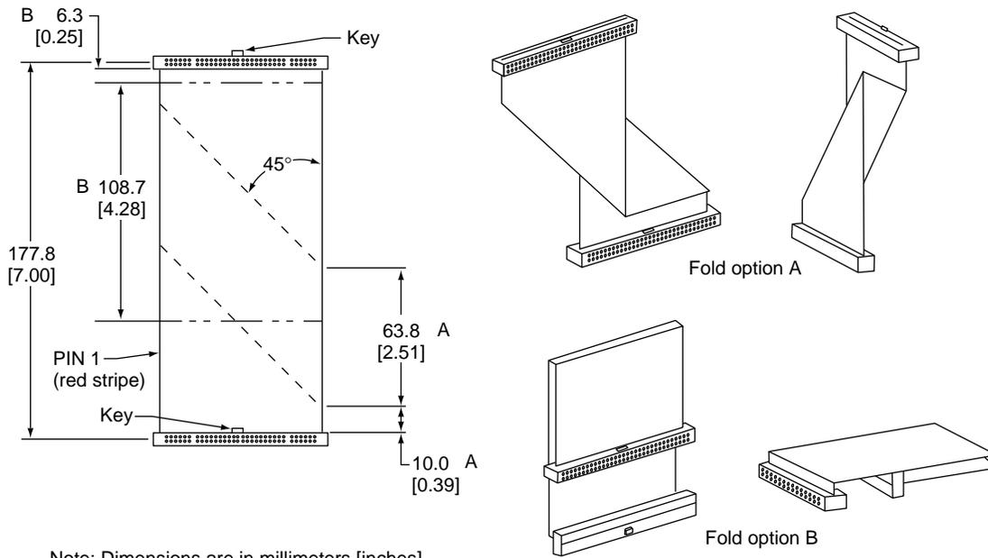
Cable fold option A, shown in Figure 4-2, is used for tower and mini-tower models such as the Power Macintosh 7500 and 8500; fold option B is used in the Macintosh Performa 6400 and all-in-one models such as the Power Macintosh 5400. Total cable length in both cases is 7 inches.
