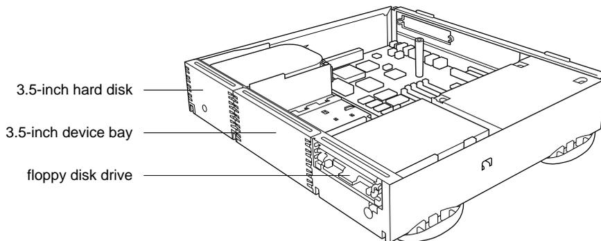
**Figure 5-2** Device locations in the Macintosh Quadra 800 computer
