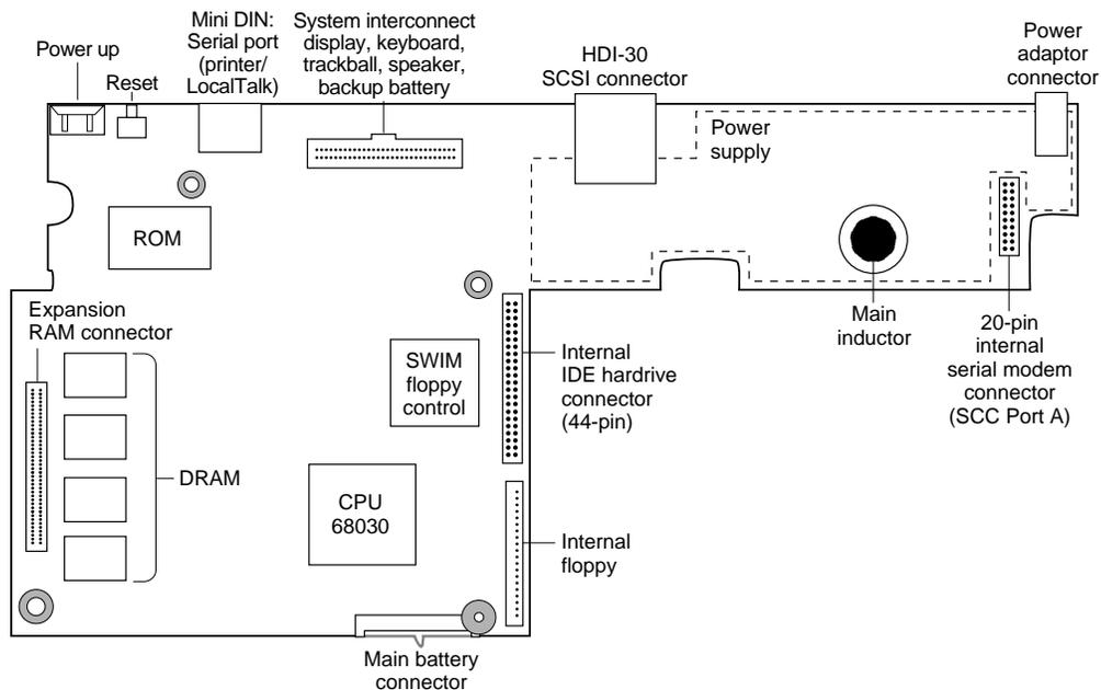
Figure 1-3 shows the locations of the supporting logic components on the bottom of the PowerBook 150 main logic board.
