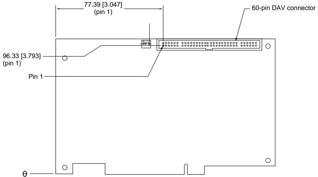
The DAV connector on the video input card provides some of the functionality of the DAV connectors found on the Power Macintosh Power Macintosh 7100 and 8100 models, and the Macintosh Quadra AV models, but it is not compatible with any of those connectors. Refer to *Macintosh DAV Interface for NuBus Expansion Cards* in *Developer Note Number 8* for more information.
