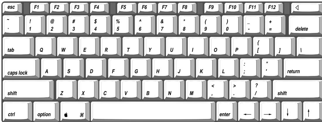
**Figure 3-4** Keyboard, ISO layout
