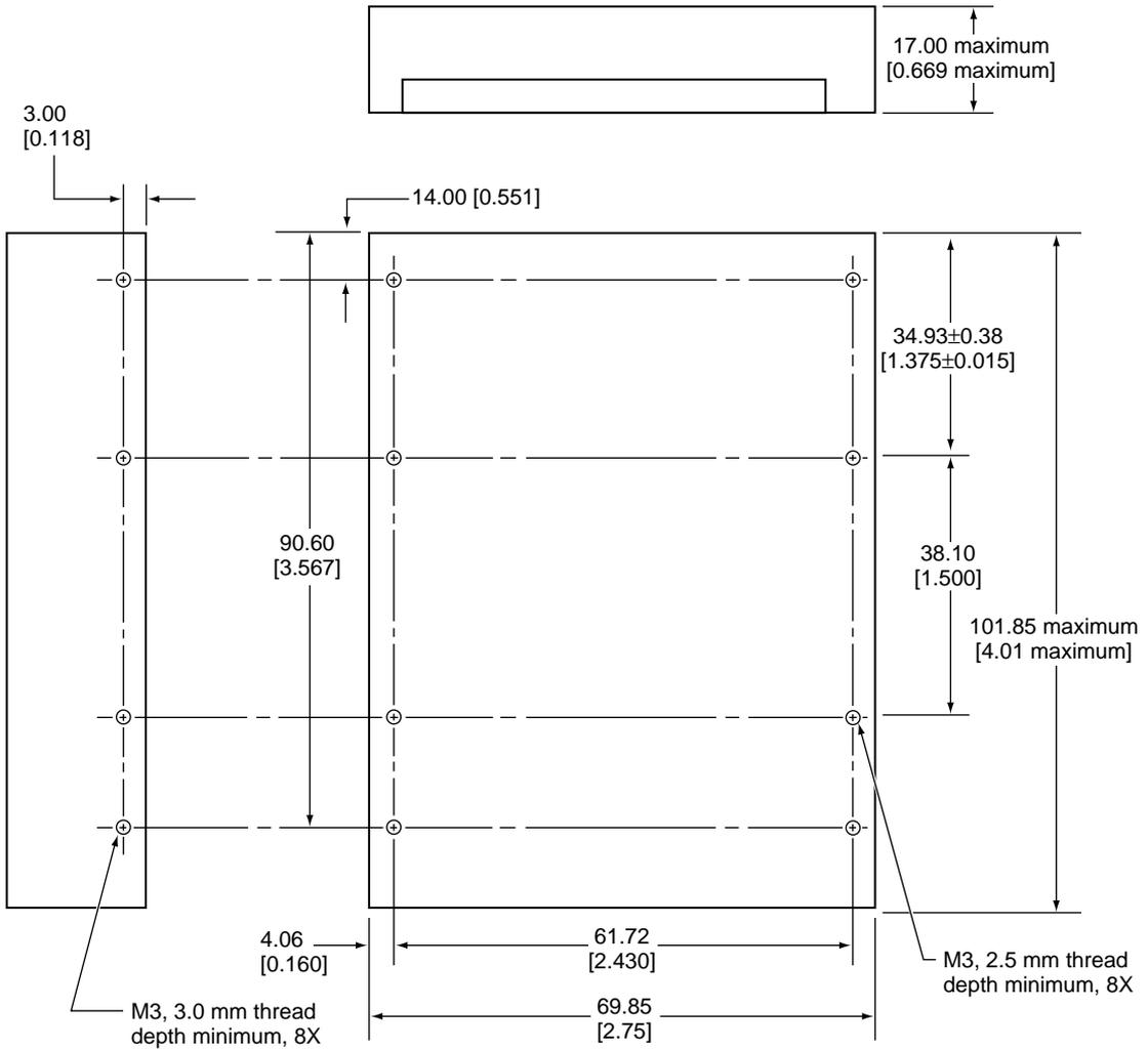
Note: Dimensions are in millimeters [inches].
