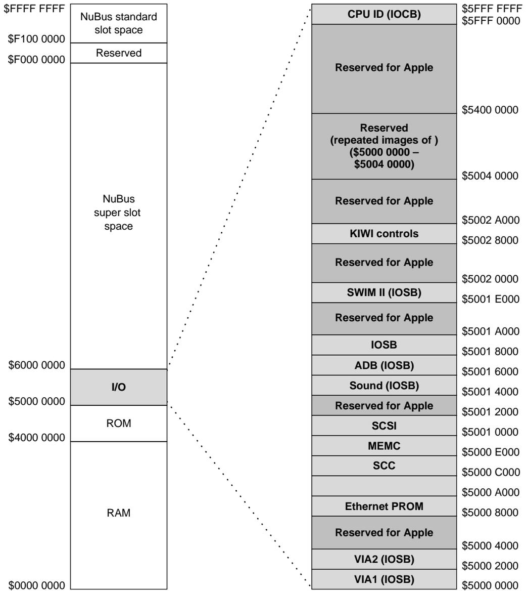
**Figure 2-5** Addresses of expansion slots
