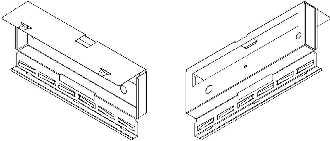
Foldout 3 is a design guide for the bezel shield used with the AppleCD 300i in the Macintosh Centris 610 computer.
