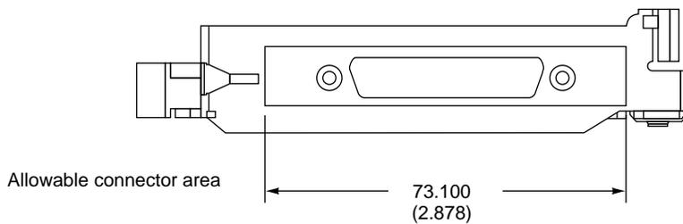
The 7-inch version of the NuBus card can be used in any Macintosh computer that has NuBus slots. Figure 3-5 shows how a 7-inch NuBus card aligns with a standard NuBus card.
