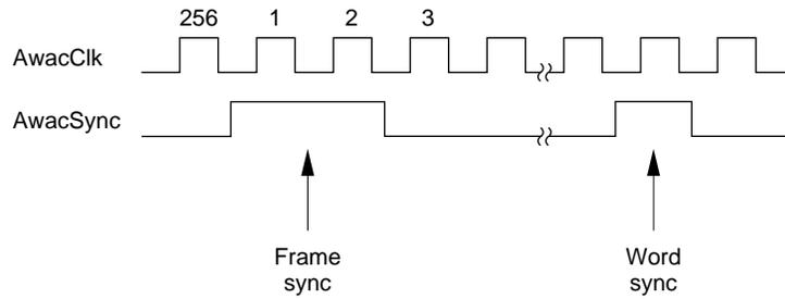
The AwacSync synchronization signals for each subframe are shown in Figure 2-3.
