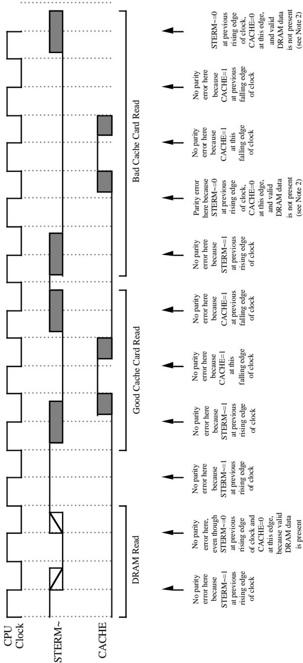
Note 1: The cycles shown in this diagram are meant to show various possible relative timings of STERM~ and CACHE, as they affect parity checking in a Macintosh IIci with parity option. These cycles do not represent actual Macintosh IIci DRAM or cache card cycles.
