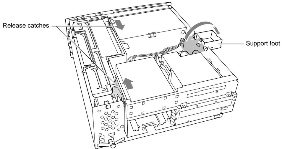
**Figure 1-4** Top chassis in open position
