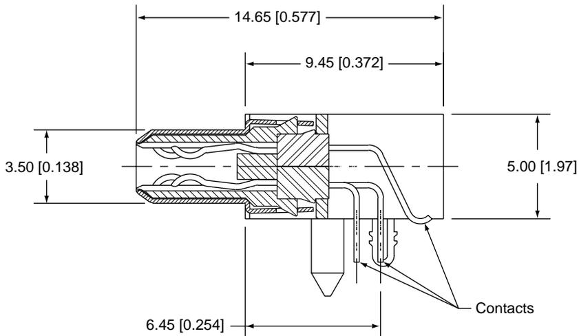
Note: Dimensions are in millimeters [inches].
