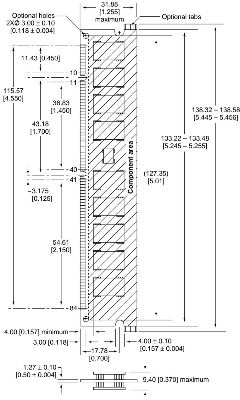
Note: dimensions are in millimeters [inches]
