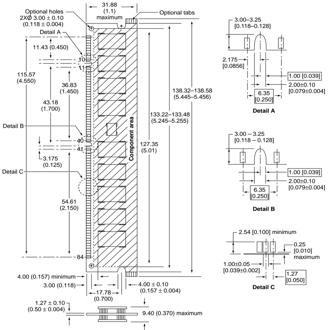
Note: dimensions are in millimeters (inches)
