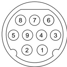
Either port can be independently programmed for asynchronous or synchronous communication formats, including AppleTalk and the full range of Apple GeoPort protocols. With external modules connected to the serial ports, the computer can communicate with a variety of ISDN and other telephone transmission facilities.
