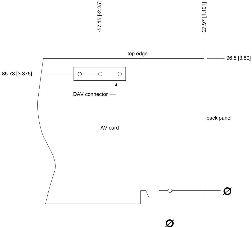
To use the Power Macintosh DAV interface, a NuBus card must have a flat ribbon cable terminating in a plug that fits the DAV connector on the AV card. Card designers should analyze the physical relations between the AV card location and possible NuBus card locations in the Power Macintosh 7100/66AV and 8100/80AV to determine the appropriate length and configuration of the card-to-card ribbon cable. When the NuBus card is adjacent to the AV card, a typical cable length is 2.5 inches.
