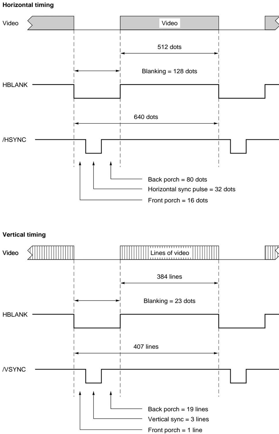
**Figure 2-5** Horizontal video timing for the Apple IIe card
