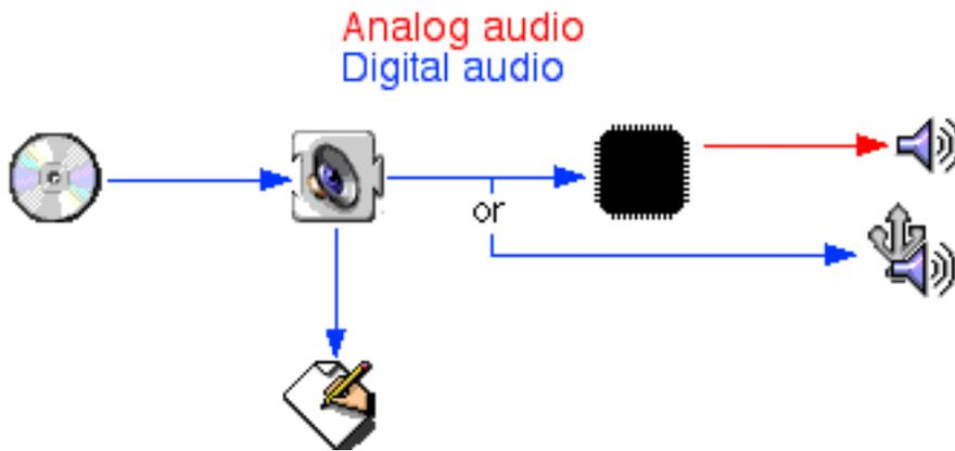
However, this also means that the CPU is now running code that plays the audio. A very minor performance penalty is extracted for this new functionality. The measured statistics are about 0.5% CPU usage on a PowerBook G3 300MHz when the sound output setting is set to 44.1 kHz. This number doesn't include the cost of the Sound Manager sound channel which is needed for the sound output.
