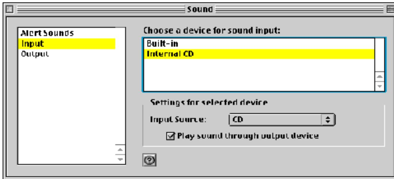
Instead of using the digital-to-analog converters built into the CD-ROM drive (which may be of questionable quality to audio purists), the audio is read as digital data, much like a normal file would be read off of a CD. This digital audio is then passed to the Sound Manager which plays it, as it would play any sound.
