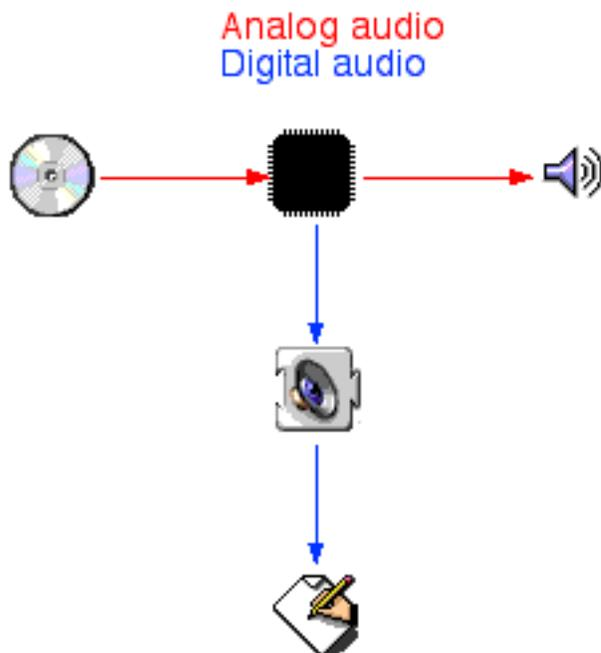
The audio data was read by the CD-ROM drive and converted to analog audio inside the CD-ROM drive.
