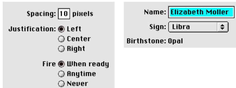
Figure 3-33 Right-alignment of dialog box item labels
