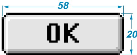
Figure 3-17 OK button showing standard push button size
