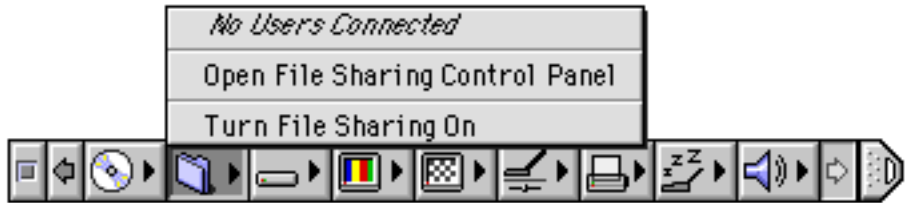
Figure 6-15 Access to a control panel from a control strip
