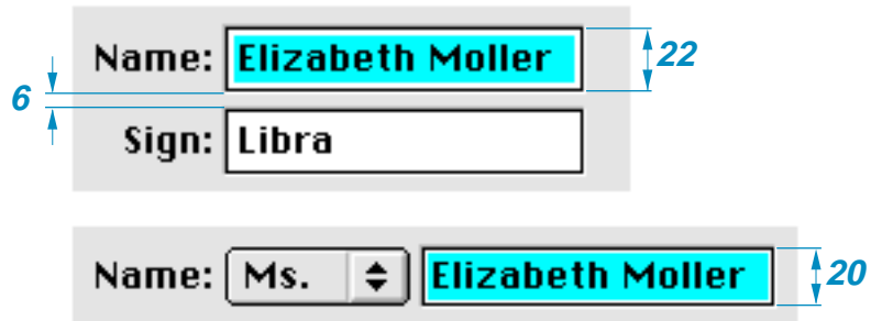
Figure 3-30 Spacing and height of edit text fields
