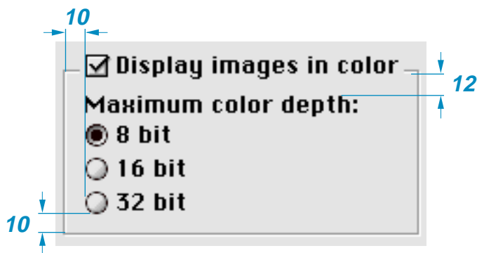
Figure 3-27 Visual layout measurements of controls in a group box
