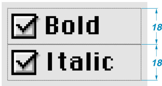
Figure 3-22 Checkbox height
