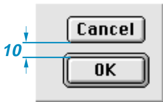
Figure 3-18 Distance between vertically stacked buttons
