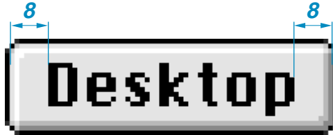
Figure 3-16 Spacing of text in a push button
