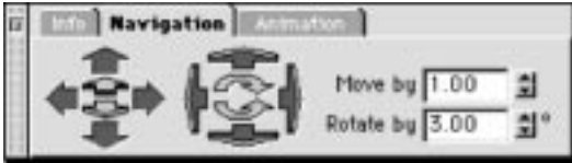
Navigation Floater - Pan, dolly, tilt, truck, crane, and roll controls for active window
