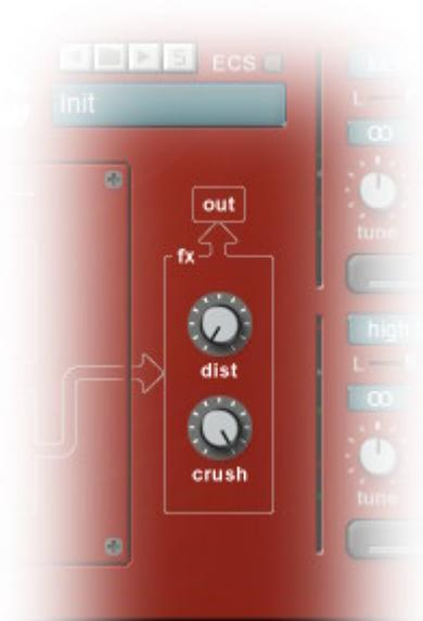
**Crush:** The Crush (BitCrusher) control enables you to reduce the bit depth of the output signal from ∞ bits (the signal is not changed) to 1.00 bits. Reducing the bit depth adds a harsh, noisy quality to the sound.
