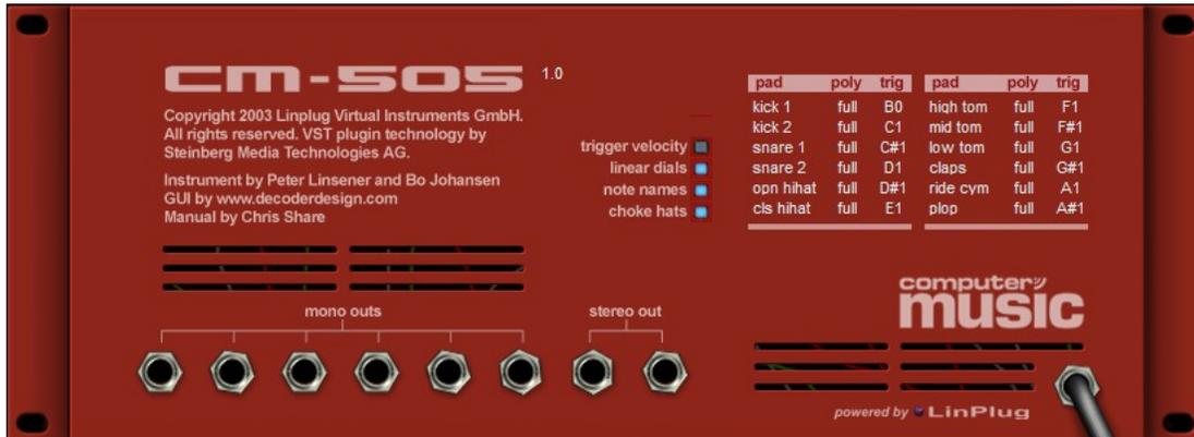
Several master controls have been located here to make the front panel less crowded, and also so that they are not changed accidentally while the CM-505 is in use. The controls located on the Rear Panel are Trigger Velocity, Linear Dials, Note Names and Choke Hats. These controls are described below:
