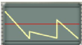
**RANDOM RAMP:** This unique shape starts each cycle by instantaneously jumping up to the new random value and then spending the rest of the cycle ramping down to minimum.
