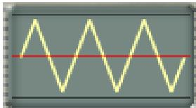
**TRIANGLE:** Similar to the Sine shape, but with a sharp (and potentially audible) change of direction at the maximum and minimum points.
