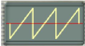
**RAMP UP:** Starts by instantaneously jumping to the minimum value and then spending the entire cycle moving up to the maximum value.
