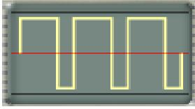
**LONG PULSE:** The inverse of the Short Pulse. Spends 75% of the cycle at maximum and 25% at minimum.
