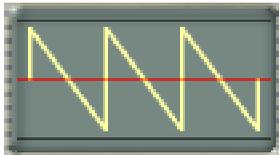
**RAMP DOWN:** The inverse of the Ramp up. Starts by instantaneously jumping to the maximum value and then spending the entire cycle moving down to the minimum value.
