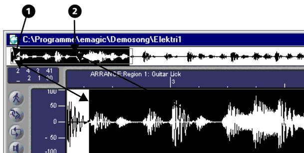
Overview display: the dotted lines box in ❶ the current section in the Waveform display window. The selection ❷ is also shown.
