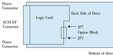
There is a choice of 2 power connections to this drive. One DC power connector is designed to mate with AMP part 1-480424 (using AMP pins P/N 350078-4). The other (3 pin) DC power connector is designed to mate with MOLEX 5480-03 (using MOLEX pins 5479). Equivalent connectors may be used. Pin assignments are shown below. As viewed from the end of the drive.
