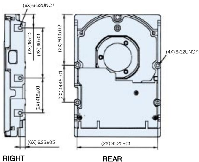
The recommended mounting screw torque is 0.6-1.0(NM) (6-10[Kgf.cm]).
