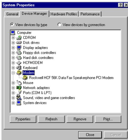
4. Click on **Rockwell HCF 56K Data Fax Speakerphone PCI Modem**
