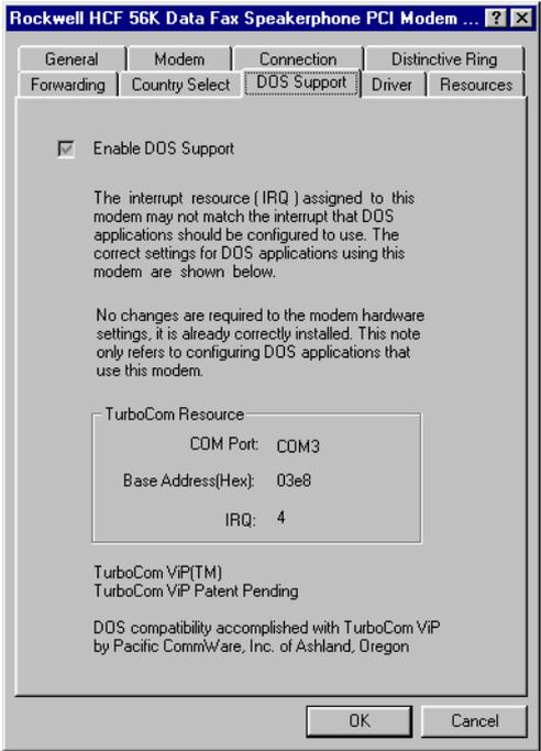
As you can see from the example above, the modem is set to use COM3 with a base address of 03e8 using IRQ4. These values are selected automatically by the TurboCom driver and cannot be modified. Use the settings displayed on this screen for your DOS based communication or online game. If you also need to modify the INIT string used by the program try one of the following:
