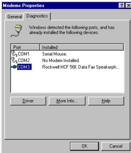
3. Click on the port the Rockwell HCF 56K Data Fax Modem is assigned to (as indicated in the previous picture).
