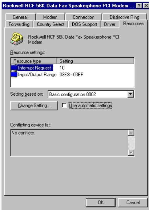
8. If you wish to change the port address that the modem is using, Click on the arrow to the right of **Basic configuration 0** and select the configuration that matches the port address you wish to use.
