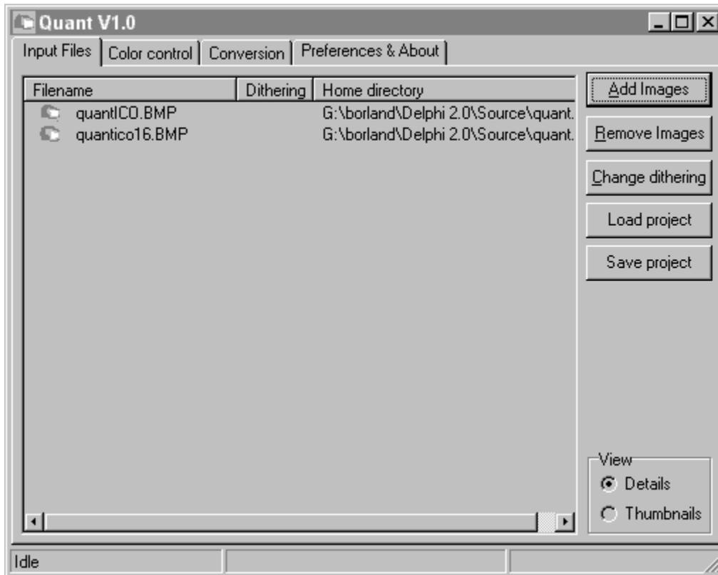
Input files menu is used to select which image files you wish to convert, you can add multiple files to the project, change dithering algorithms, remove files from the project, load and save projects.
