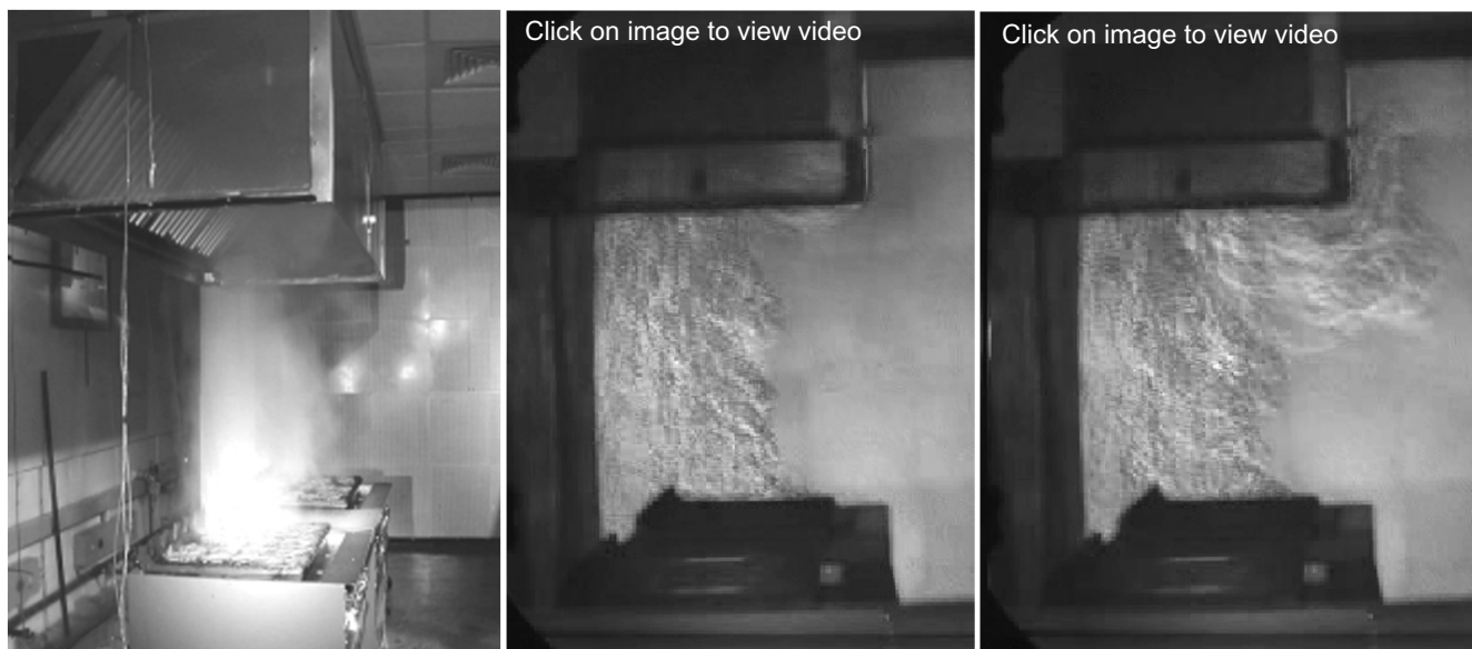
A. TEST SETUP: Two charbroilers under 2.5 m long wall-mounted canopy hood, cooking hamburgers.
