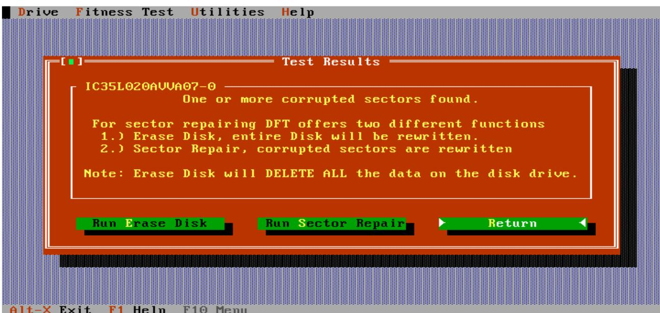
In most cases when DFT reports a media error this is because the data in a sector cannot be read due to corruption. These corrupted sectors can be recovered by being re-written, see options below.
