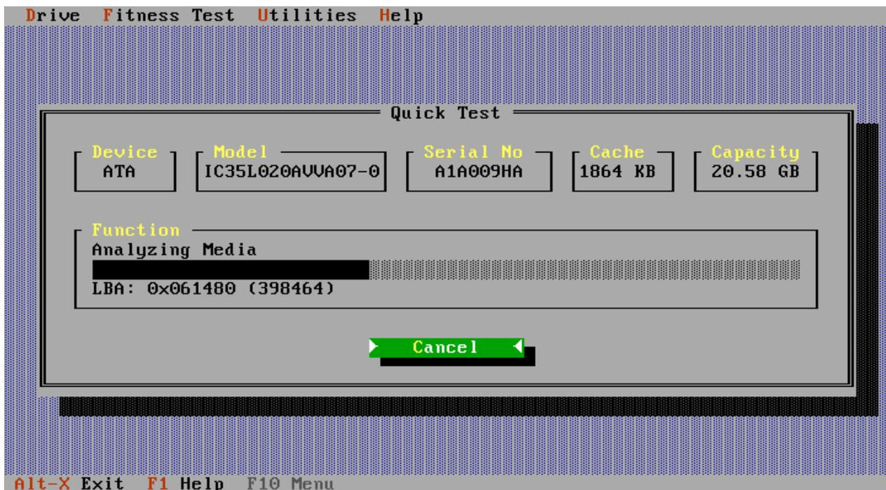
In the screen above, the DFT test is running. The active part of the test is seen to be named (Analysing Media), and the progress bar illustrates progress through the active stage. DFT execution for the Quick Test should be less than 3 minutes in most circumstances.
