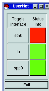
The UserNet tool from Red Hat provides a graphical interface to start and stop network interfaces.
