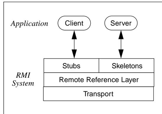
A remote method invocation from a client to a remote server object travels down through the layers of the RMI system to the client-side transport, then up through the server-side transport to the server.
