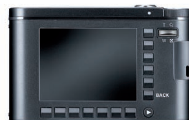
BACK: The company has engineered the use of Smart Touch buttons as shown here surrounding the LCD, to aid user navigation and selection
