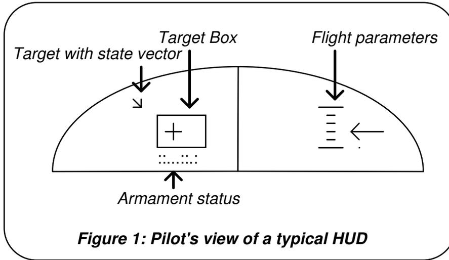
During target engagement by a high-performance aircraft, it is critical that the man/machine interface be kept very simple. There is no time to scan the cockpit for flight information in close engagements, and the pilot must watch the target at all times.
