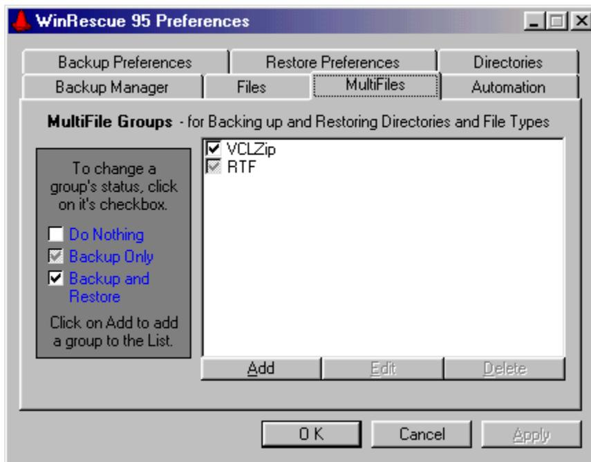
[MultiFiles Screen](#) - allows the addition of Folders and Groups of Files to WinRescue's backup. The Add button opens the [MultiFiles dialog box](#) to specify which files to include in the backup zipfile.
