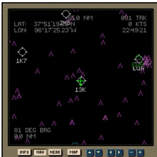
When no flight plan is loaded, the NAV map only displays the information that is toggled on in the NAV
