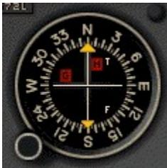
The NAV instrument is used in VOR/DME navigation primarily as an indicator of the airplane's position relative to a referenced radial on a VOR. It is also used to track localizers during ILS approaches.
