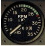
The tachometer measures the speed of the engine in revolutions per minute (rpm). The hours of operation are indicated on the number dial at the center of the tachometer. Tach time is measured by the number of engine revolutions, not by elapsed time, so an hour of engine time may not equal an hour of clock time. Only near the cruise setting will the two be equal. At slower speeds, the tach time is slower than the clock time, and vice versa at higher speeds.
