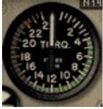
These gauges indicate the engine shaft output torque in foot-pounds.
