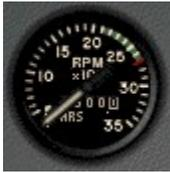
The tachometer measures the speed of the engine in revolutions per minute (rpm). The hours of operation are indicated on the number dial at the center of the tachometer. Tach time is measured by the number of engine revolutions, not by elapsed time, so an hour of engine time may not equal an hour of clock time. Only near the cruise setting will the two be equal. At slower speeds, the tach time is slower than the clock time, and vice versa at higher speeds.
