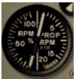
This is a dual gauge. The left side of the instrument shows the speed of the engine in revolutions per minute (rpm). The right side of the instrument shows the propeller speed in revolutions per minute.
