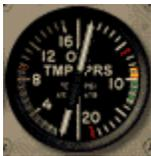
This is a dual gauge that shows both engine oil temperature and pressure. The left side of the gauge shows the engine oil temperature. The right side of the gauge shows the engine oil pressure.
