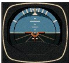
The attitude indicator is also called the artificial horizon. It shows the relationship of the nose and wings to the horizontal plane. All movements of the flight controls, such as changing pitch or bank, are done by direct reference to this instrument.
