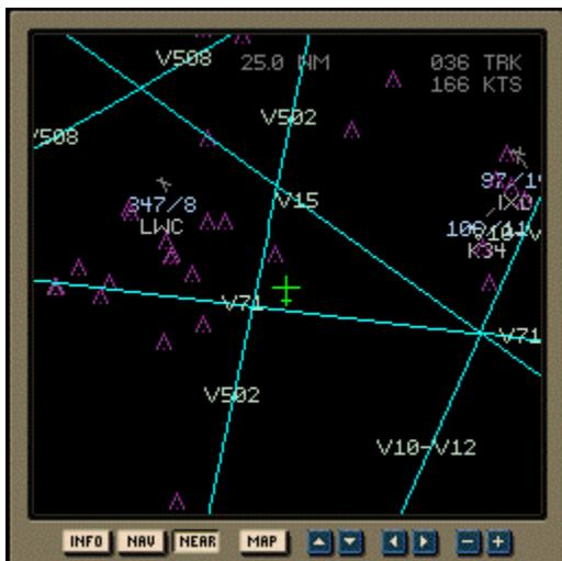
The NEAR map shows your airplane's proximity to neighboring waypoints. The type of waypoint can be selected from the NEAR menu. To toggle between the NEAR map and the NEAR menu, click the MAP button. Above each waypoint that appears on the map are two numbers separated by a slash: magnetic bearing and distance (in nautical miles) from the airplane (bearing/distance). The only other information that appears is the airplane's track and speed in the upper right corner.
