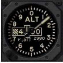
The Kollsman window within the instrument face shows the pressure plane setting which is adjusted with the knob at the lower left of the instrument. The altimeter setting at an airport is the local barometric pressure adjusted to sea level, not the actual atmospheric pressure at the station. Therefore, if the Kollsman setting is the current sea level pressure, then the altimeter reads your altitude above sea level.
