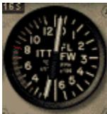
The left side of this gauge indicates the interstage turbine temperature: the temperature between the compressor and power turbines. The right side indicates the fuel flow in pounds per hour.
