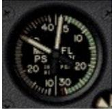
The left side of this gauge indicates the pressure inside the engine manifold in “Hg. The right side indicates the fuel flow in pounds per hour.
