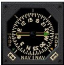
This instrument is a combined Radio Magnetic Indicator and Automatic Direction Finder. The RMI is used to track VORs. The ADF is used to track NDBs.
