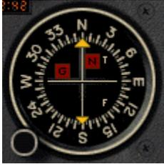
On the Baron, the HSI is the NAV 1 instrument. The NAV 2 instrument is used for VOR/DME navigation as an indicator of the airplane's position relative to a referenced radial on a VOR. It is also used to indicate the position of the airplane relative to a localizer on an ILS approach.
