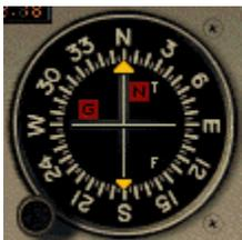
On the Bonanza, the HSI is the NAV 1 instrument. The NAV 2 instrument is used for VOR/DME navigation as an indicator of the airplane's position relative to a referenced radial on a VOR. It is also used to indicate the position of the airplane relative to a localizer on an ILS approach.
