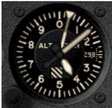
The Kollsman window within the instrument face shows the pressure plane setting which is adjusted with the knob at the lower left of the instrument. The altimeter setting at an airport is the local barometric pressure adjusted to sea level, not the actual atmospheric pressure at the station. Therefore, if the Kollsman setting is the current sea level pressure, then the altimeter reads your altitude above sea level.
