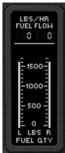
This digital display shows the fuel flow in pounds per hour for both the left and right engines.
