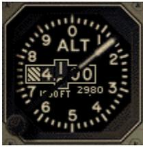
The Kollsman window within the instrument face shows the pressure plane setting which is adjusted with the knob at the lower left of the instrument. The altimeter setting at an airport is the local barometric pressure adjusted to sea level, not the actual atmospheric pressure at the station. Therefore, if the Kollsman setting is the current sea level pressure, then the altimeter reads your altitude above sea level.
