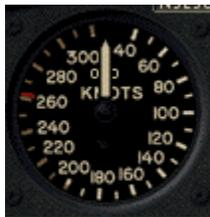
The airspeed indicator uses the ram air from the pitot tube, compares it with the static air pressure and converts it to Indicated Airspeed which is displayed on your airspeed indicator. Modern airspeed indicators show knots on the outer scale and mph on the inner scale. There are three definitions of airspeed:
