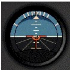
The attitude indicator is also called the artificial horizon. It shows the relationship of the nose and wings to the horizontal plane. All movements of the flight controls, such as changing pitch or bank, are done by direct reference to this instrument.
