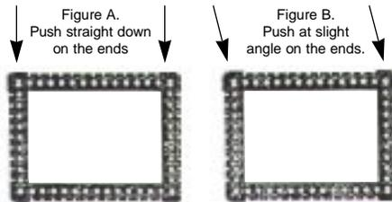
5. Put the structure on a firm surface and press straight down like in Figure A. If you do this correctly, the structure should not move. Now change from pushing straight down and push slightly to the side as shown by arrows in figure B.
