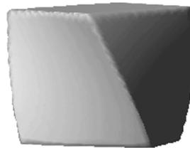
*figure 17.19: Cube with +25% Twist Applied*
