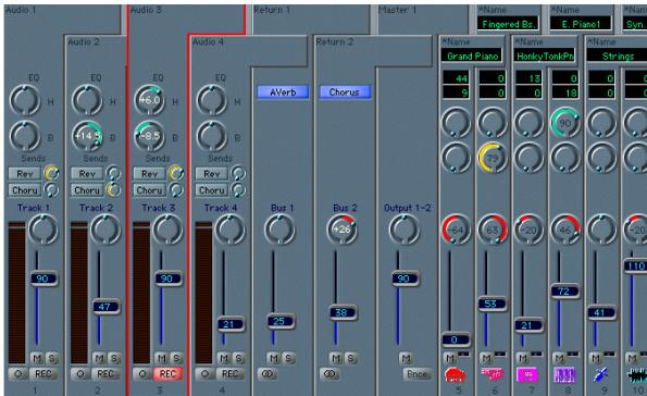
If you use a GM-compatible tone generator connected to your computer, you can control its functions remotely from the Mixer window. Selecting sounds, controlling the volume, or adding chorus or reverb etc. is as easy as can be. Logic Fun also supports the GS- (Roland), or the XG format (Yamaha). With these devices, more sound and effect parameters can be remote-controlled, for example, the filter frequency.
