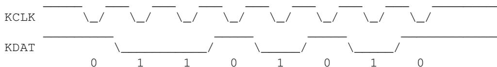
In the next example, the B key is released. The keycode is still \$35, except that bit 7 is set to indicate "key-up," resulting in a code of \$B5 = 10110101. After rotating, the transmission will be 01101011:
