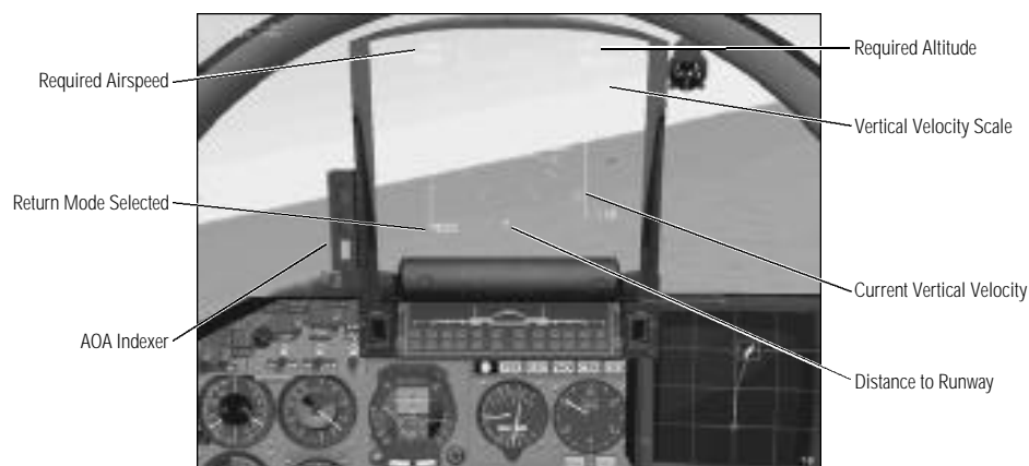
4-6: The ПОО -(LNDG) Landing Submode with ILS
