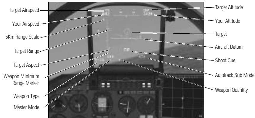
4-15: Autotrack Symbology with Radar Lock
