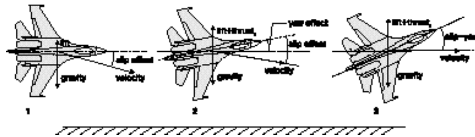
Figure 5-3: Slip Angle
