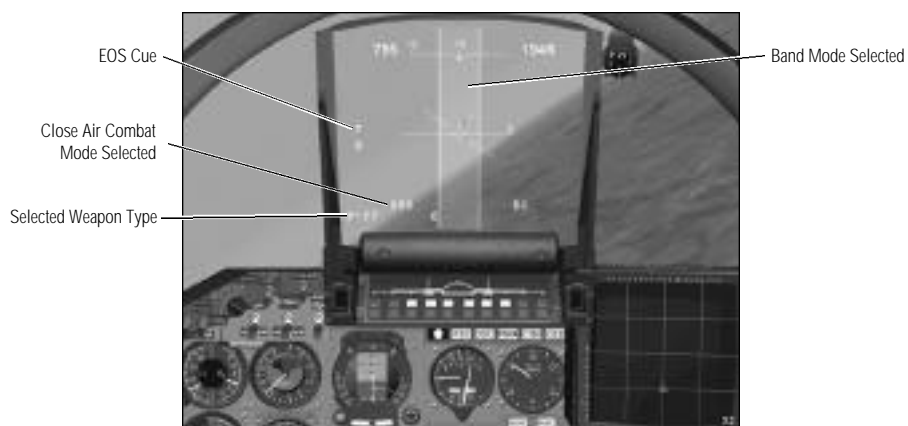
4-10a: The Vertical Scan Mode Close Air Combat Symbology
