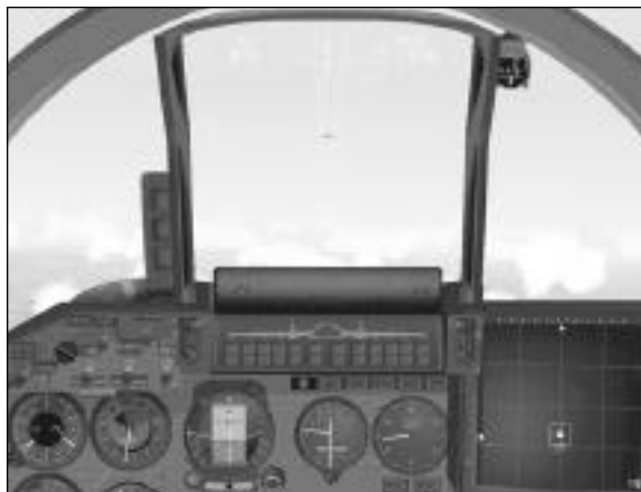
6-3: The Autotrack HUD Symbology (Range > 1400 meters)
