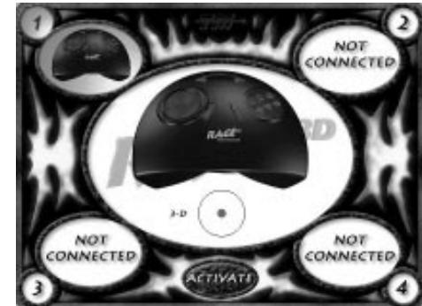
To test another control (if more than one Rage game pad is installed), leave the other controls alone and press a button on the new control until it becomes the active control in the Activator panel.
