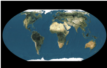
Earth surface image mapped onto a 9-km digital elevation model and rendered (in parallel) at 3000x2400 resolution using a Wagner IV equi-areal projection. Image provided by Tom Crockett, ICASE.
