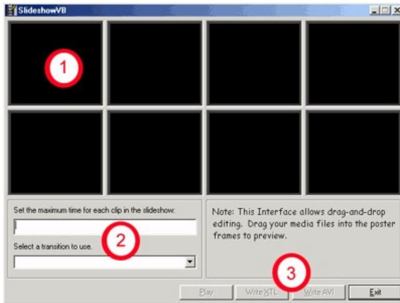
Once the application is loaded, you can begin inserting media into the cells. Starting in the upper left hand cell, work your way across the app by dragging and dropping video files into each of the cells.
