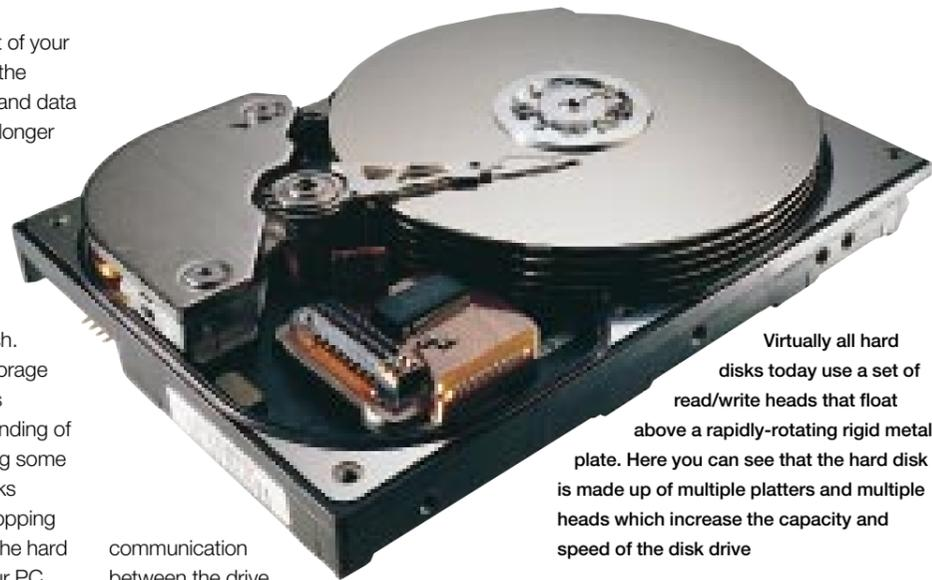
Virtually all hard disks today use a set of read/write heads that float above a rapidly-rotating rigid metal plate. Here you can see that the hard disk is made up of multiple platters and multiple heads which increase the capacity and speed of the disk drive
