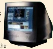
NEC's 15in multimedia monitor offers more than just a built-in pair of speakers. For a start, it uses a new type of screen called ChromaClear, which has elliptical phosphor dots that are arranged in staggered vertical lines, rather than in the usual triangular pattern. This minimises the black space between dots and increases colour depth and saturation.
