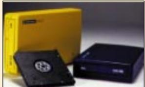
The Xyratek MaxIT is an external removable hard drive for use with both PCs and Macs. The bad news is that it's a SCSI device, which means that your PC must have a SCSI card before you can use it, although these are relatively inexpensive and easy to fit. The good news is that, once you have one, you can use several SCSI devices at once and, with Windows 95, installation is simply a matter of plugging them in.
