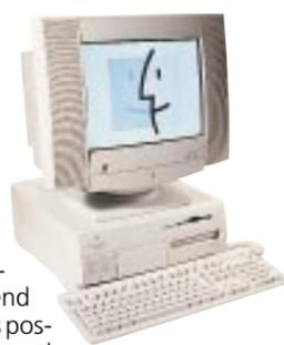
Inside there are several other differences too. The processor is a high-end PowerPC 604 running at 132MHz. It is possible to upgrade this processor, so the 7600/132 can grow to meet your future needs. Also, the machine has three free PCI expansion slots, which can accommodate a multitude of add-in cards.
