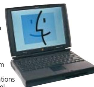
The PowerPC 603e processor makes its third appearance in this feature, but this time it's the lower-speed 117MHz version. This is fine for use in notebooks because they are generally used for less demanding tasks than their desktop counterparts.
