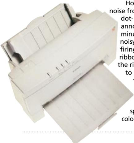
This makes them virtually silent, but also accounts for their high running costs: ink cartridges are expensive although prices are falling. The paper comes out of the printer with wet ink on it and, unless you leave each page to dry for a few seconds, it will smudge if you touch it. Inkjet technology, which is capable of producing high-quality output, thus carries its own
