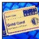
The Gold Card Global is approved for use in more than 20 countries and it will work in all of them, thanks to the supplied country-switching software. The 33.6Kbits/s card also works as a Group 2 fax and has 2Mb of flash memory for handling upgrades to new communications standards.
