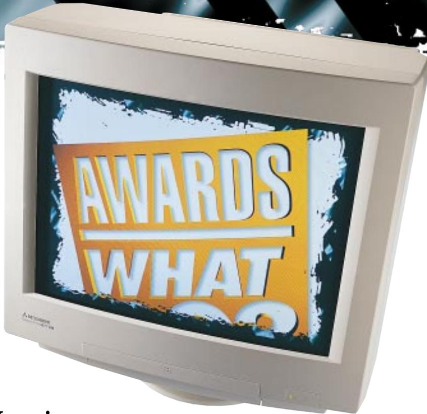
the name may sound reminiscent of Sony's Trinitron and, in fact, this is Mitsubishi's version of the Trinitron, following a technology exchange deal with Sony. The external characteristics of the two screens are the same, both being flat in the vertical plane, giving a very flat image.
