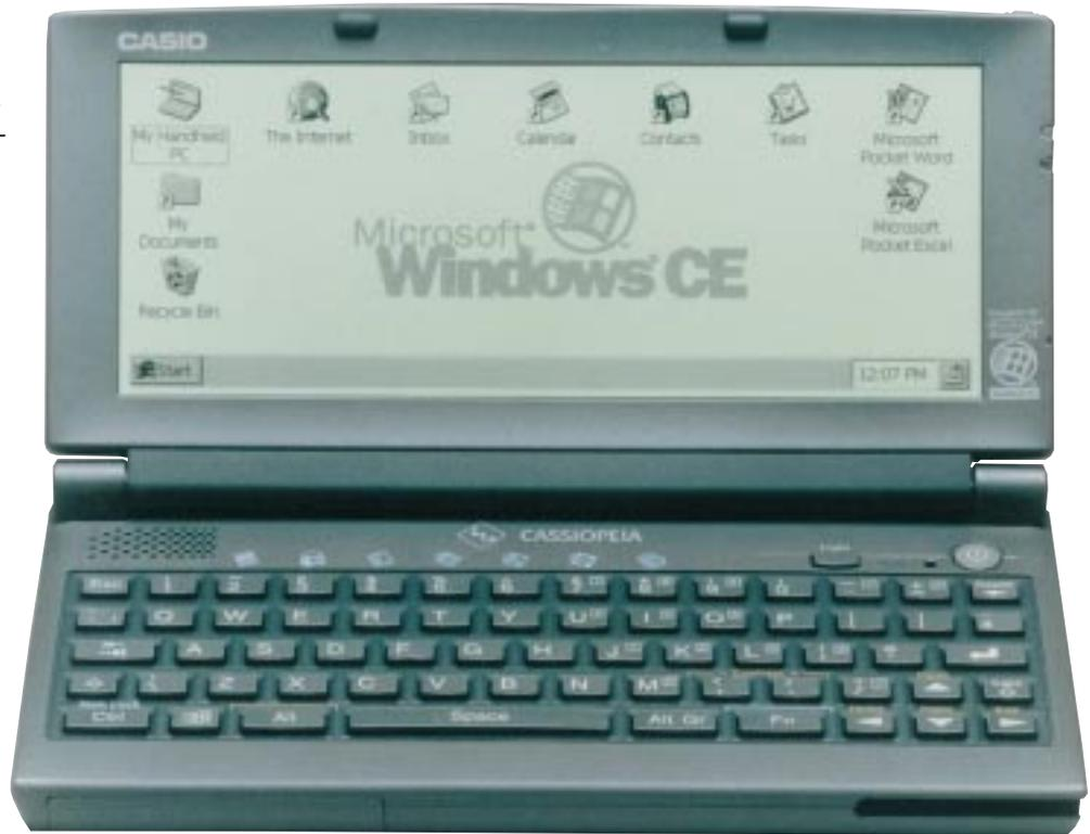
nected to a Casio digital camera for downloading images for use in documents and e-mails. The Cassiopeia also has a couple of LEDs on the edge of its lid for silent alarms but both HPCs have a built-in speaker loud enough to disrupt most meetings.
