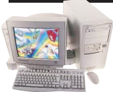
**E**vesham Micros was one of three manufacturers to send in a PC powered by the latest 300MHz Celeron processor. There is no on-board Level 2 cache on these chips, but the higher clock speed should give a performance hike.
