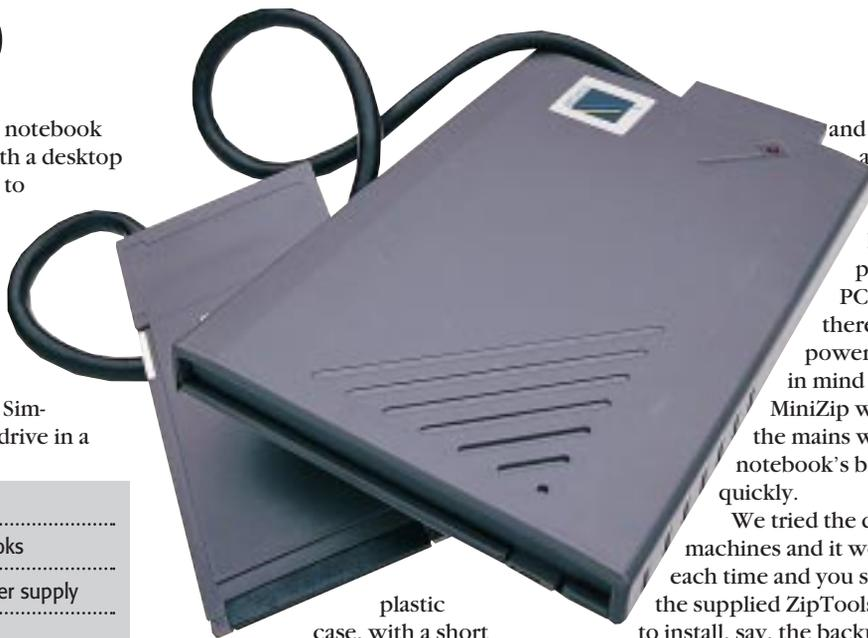
and the drive simply appears as another one in My Computer. Power is supplied through the PC Card slot, so there's no separate power supply but bear in mind that using the MiniZip while away from the mains will drain your notebook's battery more quickly.
