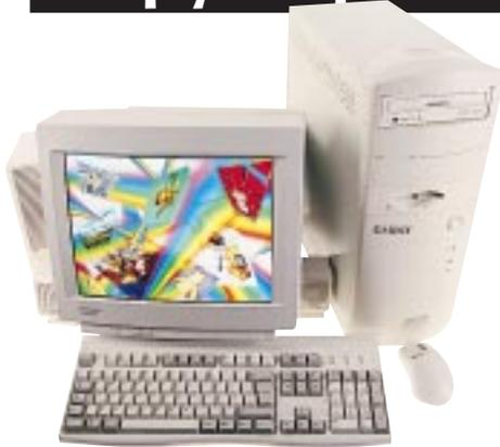
**T**he Simply Computers Multimedia 210P came with one added extra that none of the other machines featured – an Orchid Righteous 3D Voodoo 1 graphics accelerator card. But the rest of the spec was pretty similar to the other 266MHz Celeron systems in the test, with 32Mb of RAM and a 4.3Gb hard drive.
