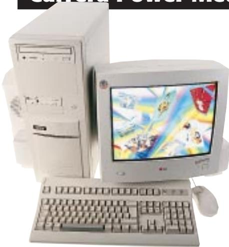
**C**arrera supplied a 300MHz processor in its PC, the most powerful Celeron chip available at the time of this test. The rest of the spec is one of the best too, with 64Mb of RAM and a 4.5Gb hard drive. It also uses ATI's brand-new Xpert 98 graphics card, which benefits from a generous 8Mb of RAM.
