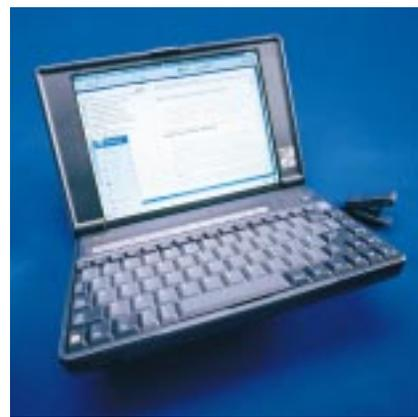
A quick comparison between the Tecra and the Hewlett-Packard Omnibook reveals plenty of similarities. Like the Tecra, the Omnibook is powered by a Pentium 166MMX processor, it has pipeline burst secondary cache (512Kb rather than 256Kb though), a 2.1Gb hard disk and an active-matrix screen. There are some differences too, including the fact that the Omnibook comes with 16Mb of RAM, not 32Mb, as standard, and while it can be used with a CD-ROM drive, this is external only and sold as an option.
