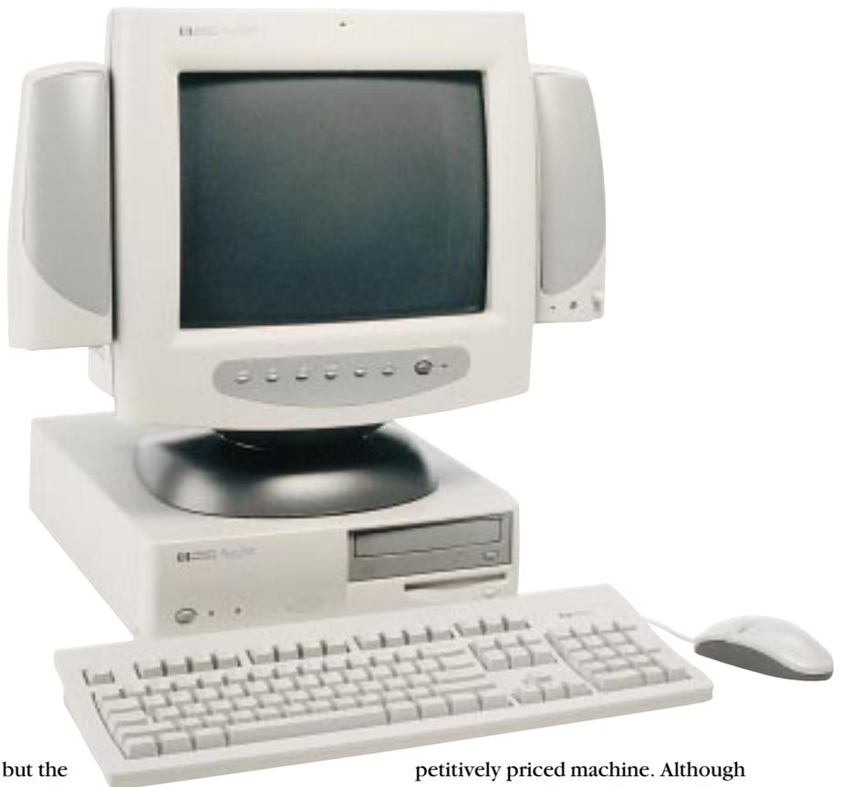
There's an internal 33.6Kbits/s ISA modem in one of the two expansion slots and the graphics adaptor and sound hardware are integrated onto the motherboard. This leaves the PCI expansion slot free in case you want to fit a 3D accelerator card or similar accessory. The only other internal upgrade you can make is to add a second memory module to increase the 16Mb of RAM supplied as standard to a more versatile 32Mb. Other accessories can be connected to the two USB ports on the back of the case.
