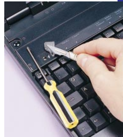
Screws can be hidden under adhesive labels
