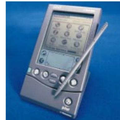
If you're looking for the ultimate in portability the US Robotics PalmPilot is the answer. It's small enough and light enough to carry in a shirt pocket and makes even the Psion 3c look clumsy. However, there's no room for a keyboard, most of the front surface being occupied by a 160x160 pixel screen. This does not normally require a backlight, though one is provided.
