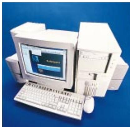
MJN's 233M Ex is more traditional in design than Compaq's Presario but it's a worthy competitor thanks to its higher specification and cheaper price. The processor is the same, a 233MHz Pentium MMX, but in this case is supported by a far more useful 64Mb of RAM and twice as much cache RAM.
