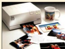
The Fotofun printer is a thermal dye-sublimation printer, which refers to the way in which it transfers an image to the page. It uses a three-colour film that is wound onto a roller and prints are made in three passes – one for each colour. The ribbon is only used once and is progressively wound on as prints are made. Using the standard print kit, consisting of a ribbon and 36 blank 'photos', a single print works out at about £1.20. Kits are also available for printing postcards and even mugs.
